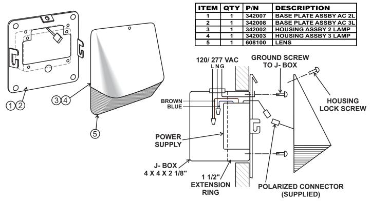
If product is supplied assembled, to separate housing and base remove #6-32 lock screw at top of housing and move housing up and out to release pins.
