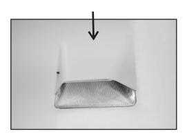
5. Locate housing pins in slots provided in base, move downwards to lock & secure with one #6-32 screw provided. Apply AC line power, check the LED Status Light is illuminated GREEN and press the PUSH TO TEST to check lamp operation in emergency mode
