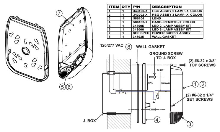
Product is supplied assembled. To separate Housing and Base, remove two #6-32 screws at top of housing and back out two #6-32 set screws on each side.
