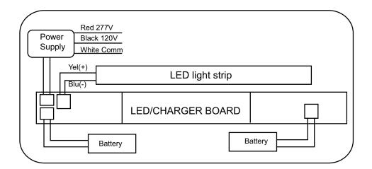
Note: Cap off the **UNUSED** input lead. Failure to do so can cause an unsafe operating condition.
