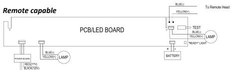
**CAUTION:** DO NOT connect YELLOW and BLUE remote leads together. Please also ensure remote head positive (+) lead is connected to COMBO unit's yellow lead (+) and remote head negative (-) lead is connected to COMBO unit's blue lead (-).
